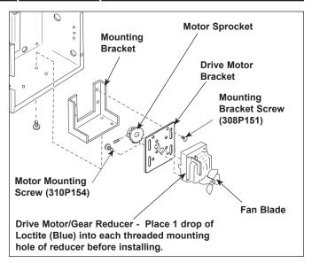
Figure 10. Replacing Drive Motor and Fan Blade
